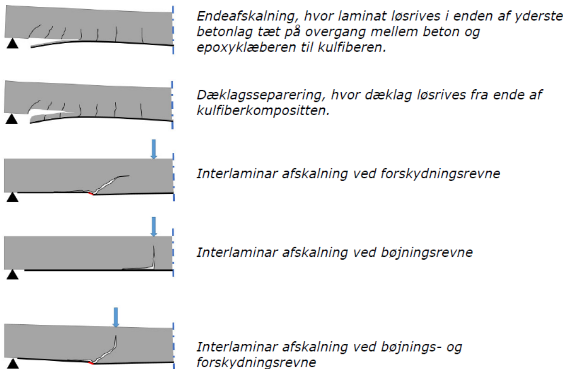
Figur 11. Forskellige brudformer for delaminering.
